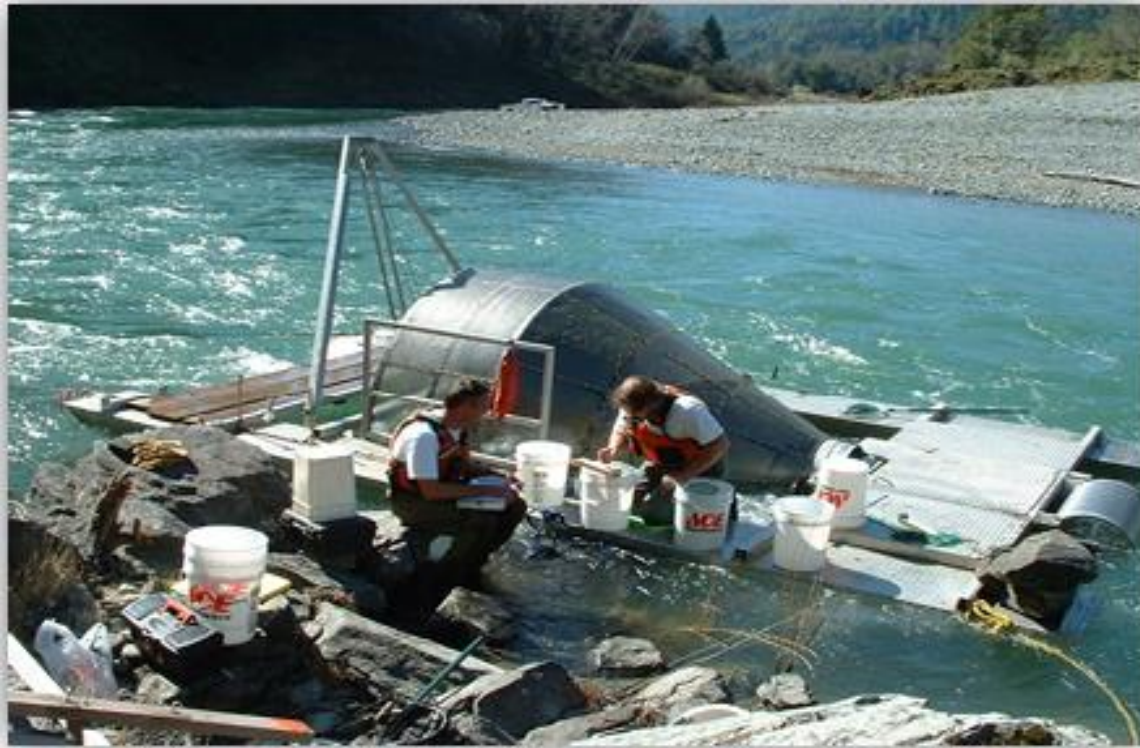
Rotary Screw Trap on the Trinity River. Credit: USFWS
